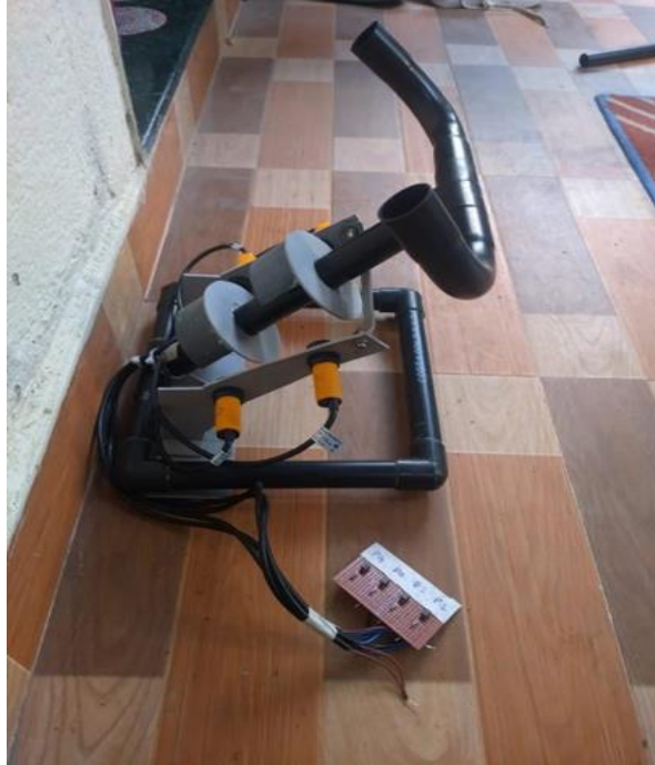
Fig. 5 Steering column with Proximity sensors
