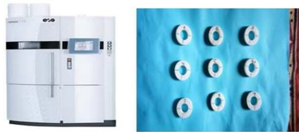
Fig: 1 Rapid Prototyping machine at Department of Mechanical Engineering Osmania University Hyderabad and sintered PA2200 prototypes
