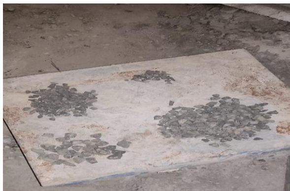
Fig. I Sieve Analysis sample for Coarse Aggregate
