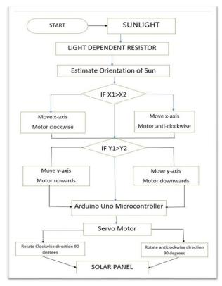
The *Flowchart* of process attached below demonstrates the progression of procedures taken during the design and operation of our project.
