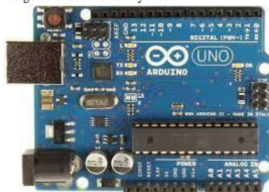
Figure 1, Arduino Uno Rev 3 microcontroller
