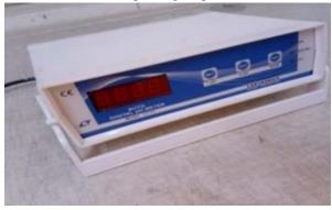
Viscosity determination: Viscosity of the formulation was determined by Brookfield Viscometer at 100 rpm, using spindle no 7.
