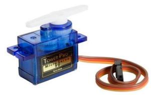
A Servo motor is a type of motor that consists of a control circuit that provides feedback on the current position of the motor shaft, this feedback allows the servo motors to rotate with great precision.
