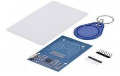
Radio Frequency Identification is a type of wireless communication that uses electromagnetic or
