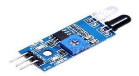
An infrared (IR) sensor is an electronic device that measures and detects infrared radiation in its surrounding environment and also can be used for motion detection.
