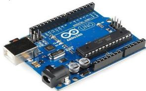
Arduino Uno is a microcontroller board based on 8-bit ATmega328P microcontroller. Along with ATmega328P, it consists other components such as crystal oscillator, serial communication, voltage regulator, etc. to support the microcontroller. Arduino Uno has 14 digital input/output pins (out of which 6 can be used as PWM outputs), 6 analog input pins, a USB connection, A Power barrel jack, an ICSP header and a reset button.
