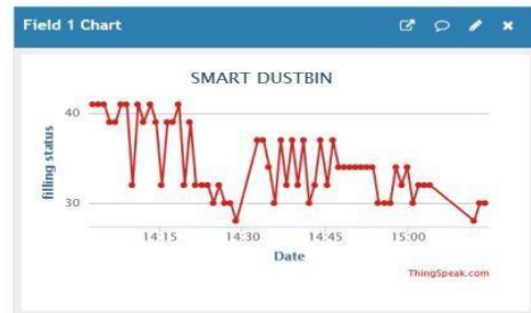
Fig. 6(a). The curve represents the filling status of the bin in the Thingspeak IoT platform for a few hours during the experimental period
