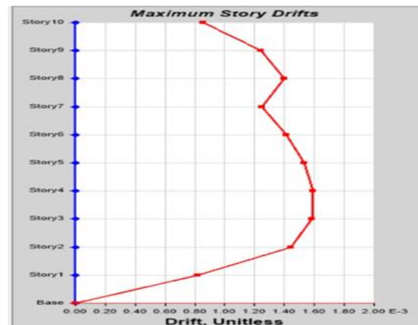
Fig.9. Model-3 (Graph of storey drift vs storey)
