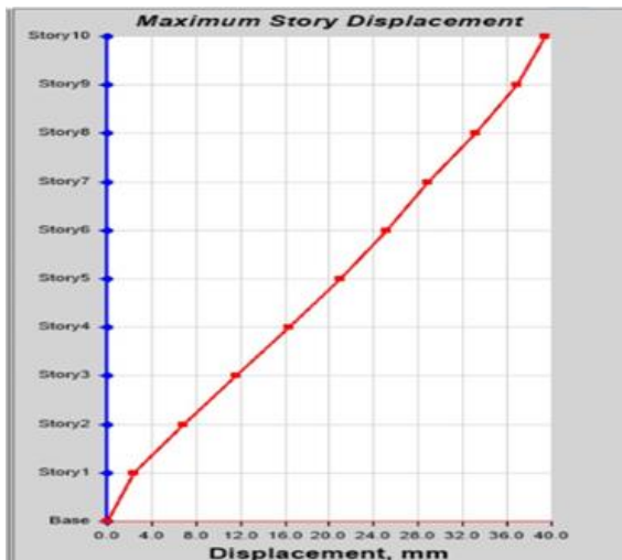
Fig.6. Model-3 (Graph of storey displacemet vs storey)
