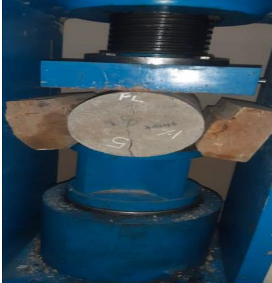
Figure 3: Split-Tensile Strength Test
