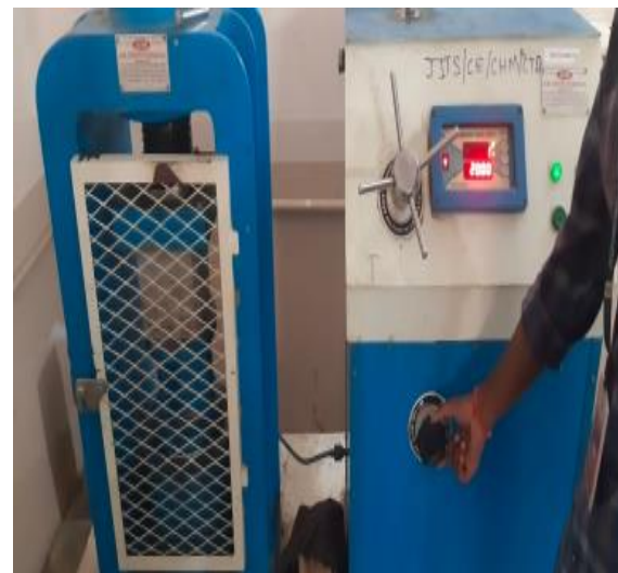
Figure 2: Compressive Strength Test
