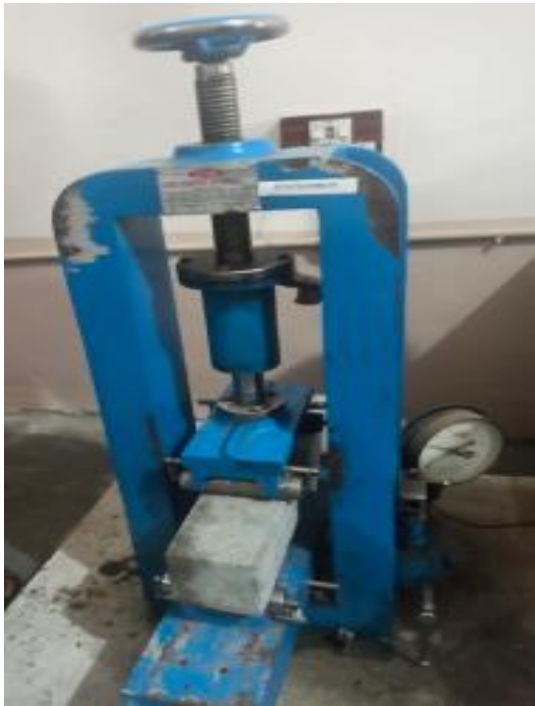
Figure 4: Flexural Strength Test
