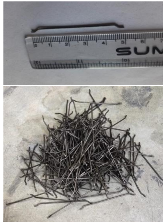
Figure 1: Hooked end steel fibers
