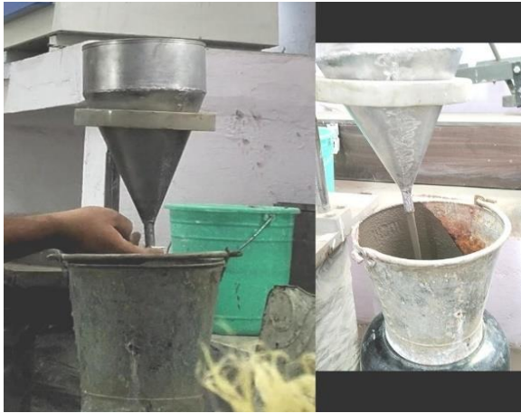
Fig.3.5 The flow cone is used to determine the flow value
