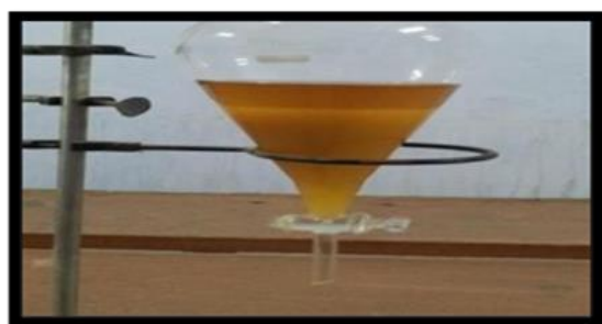
Fig. No.2 Separation of oil and glycerol, Biodiesel
