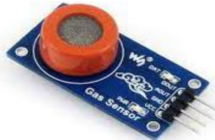
Fig. 6 MQ3- Alcohol Sensor
