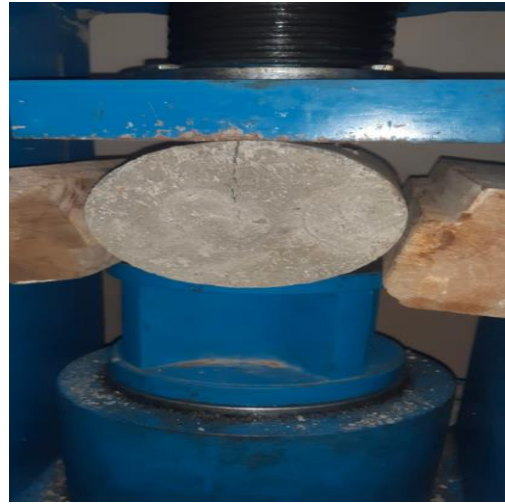
Figure 2: Split-Tensile Strength Test
