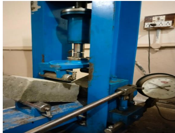
Figure 3: Flexural Strength Test
