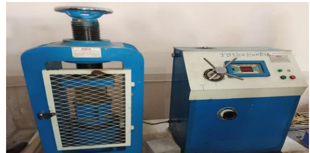
Fig 4.5 Compression strength test
