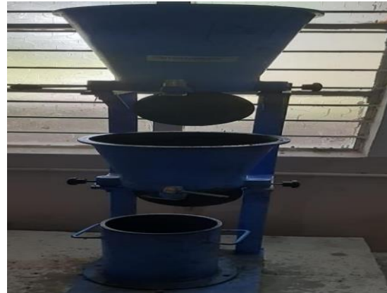
Fig 4.2 Compaction Factor Test
