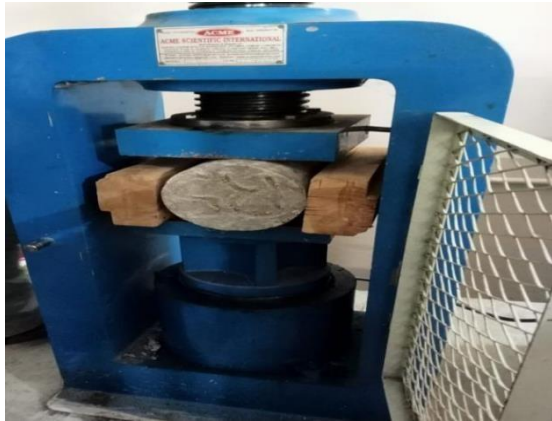
Fig 4.6 Tensile strength test
