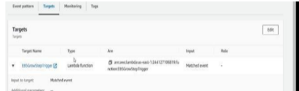
Fig 5 Event targets that are connected with Lambda Function
