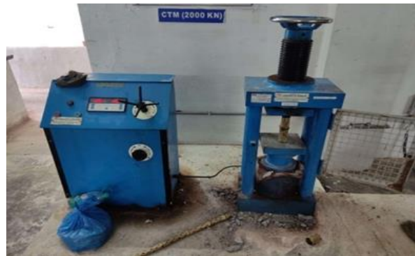
Compressive strength test of the bamboo specimen in
