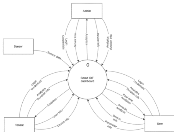
Fig.2 Represents the level-0 data flow diagram which is the visual representation of the information flow through a process or system.
