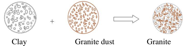
Fig 3.5 Change in the particle gradation of clay soil with addition of granite
