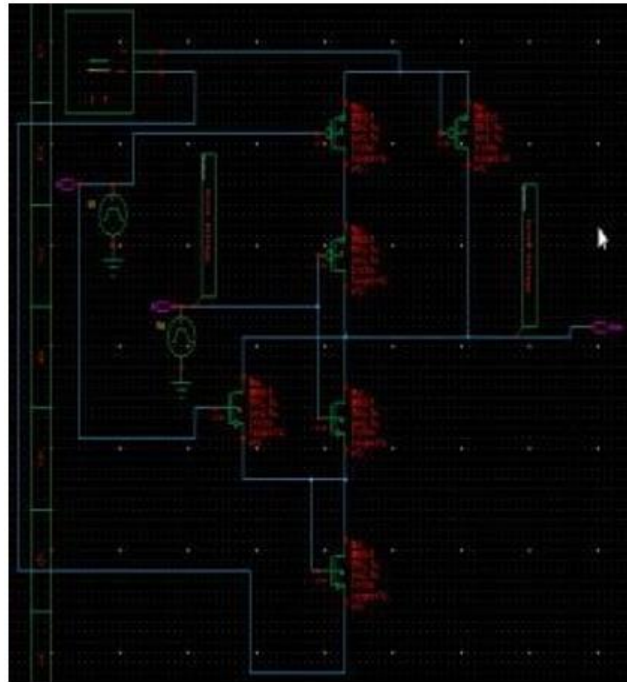
Fig. 7: Schematic of NOR Gate using 2PASCL
