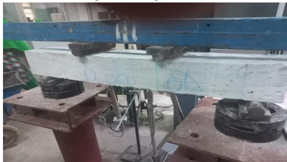
Fig 12. Failure of beam
