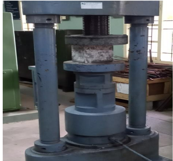
Fig4. TESTING OF CUBE compressive strength of concrete at the age of 7, 14 & 28days.
