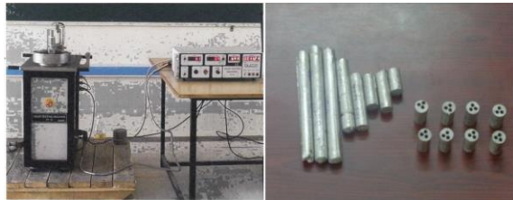
Fig. 2 Ducom TR- 20 LE with Controllers Fig. 3 Wear Test Specimens
