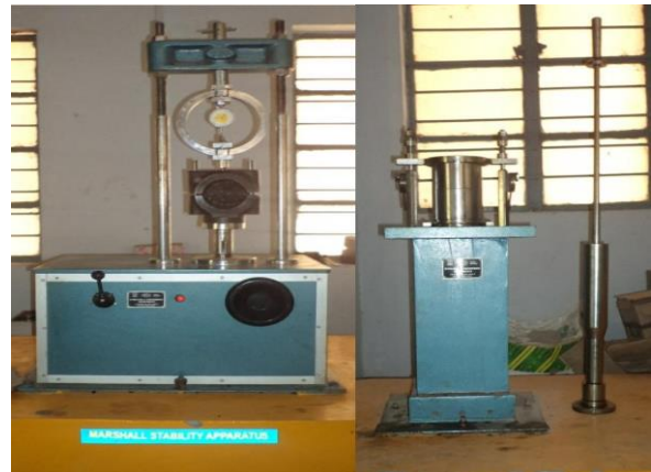
Fig.: 6.1. Marshall Test setup
