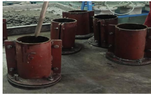
Fig 6.1 Preparation of Cylinder mould
