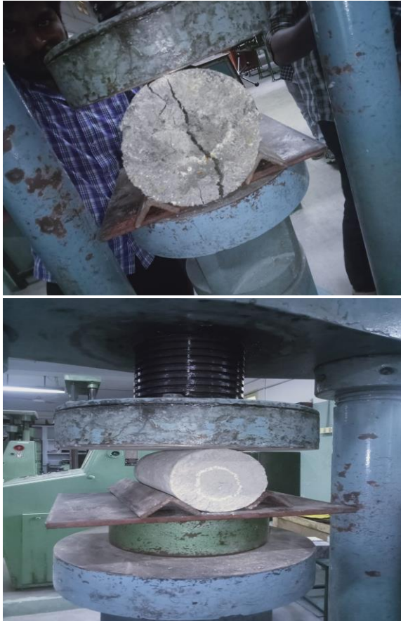
Fig 6.3 Split tensile strength test of Oyster shell powder concrete
