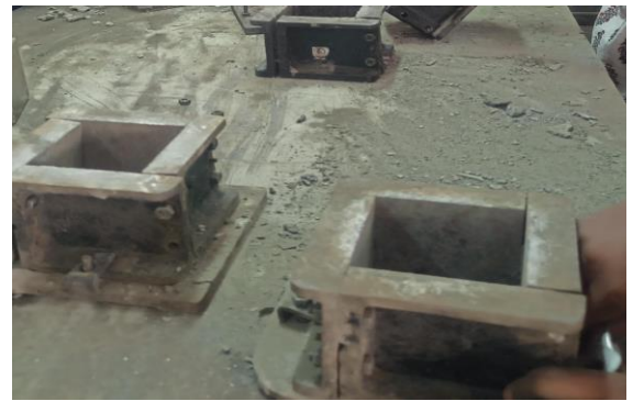
Fig 5.3 Mould preparation for cube specimen
