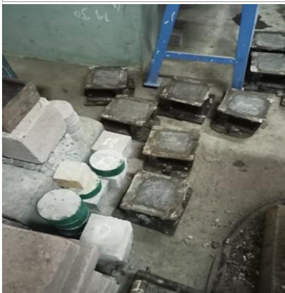
Fig 5.6 Casting of Oyster shell powder concrete
