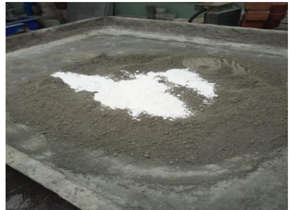
Fig 5.4 Oyster shell powder mixing of concrete
