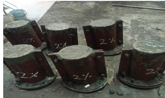
Fig 6.2 Preparation of Cylinder concrete
