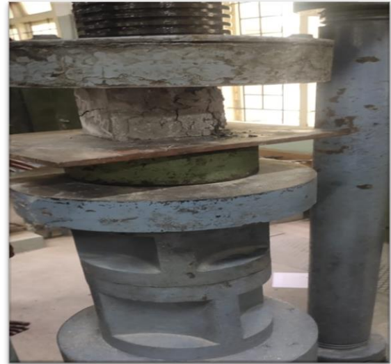
Fig 5.2 Compressive Strength Test for Conventional Concrete
