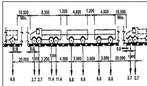
Fig 3 IRC Class A loading
