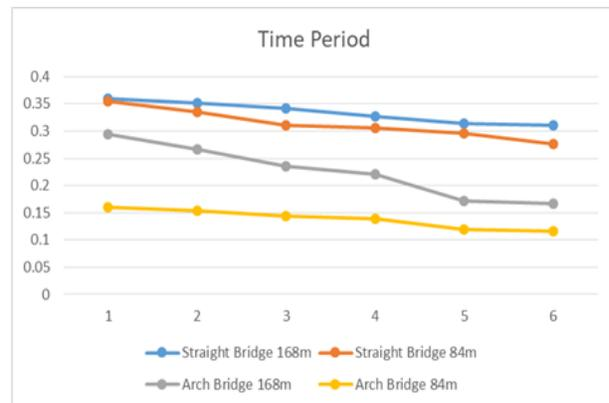
Graph 2 Time Period for Straight And skew (arch) Bridge for 168m and 84m
