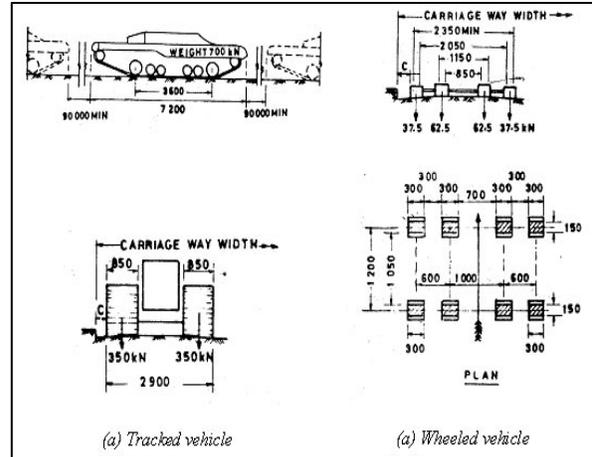
Fig 2 IRC Class AA loading
