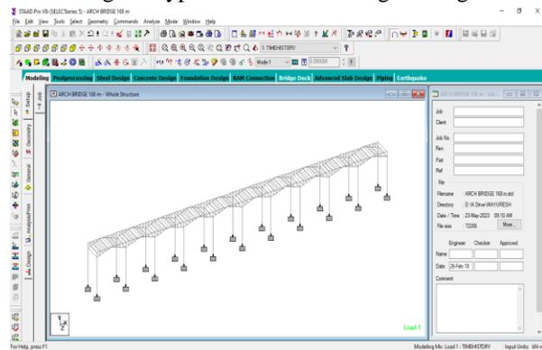
Fig. 7: Typical Model for skew (arch) Bridge
