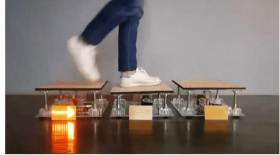
Fig 4: Design of Kinetic-Energy Harvesting Floors
