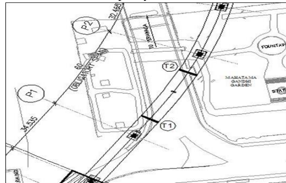
Fig 4: Trestle locations for proposed erection scheme
