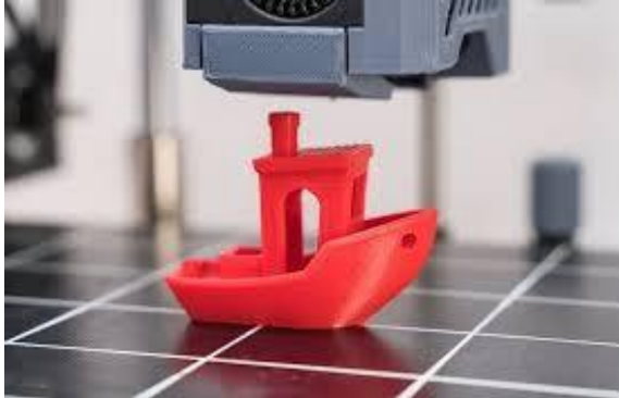
Fig. 8: A 3D printer creating a plastic boat
