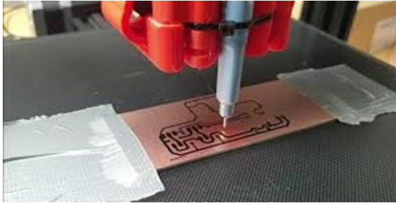
Fig. 3: Modern 3D printing technology in use, producing a sheet of PCB
