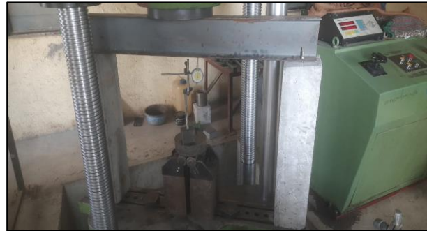
Fig 3 Initial Reading of the deflection is 5.55 mm for load 163 kn
