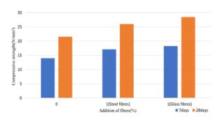
Compressive strength of normal concrete is  $14.00 \, \text{N/mm}^2$  At 7 days and  $21.16 \, \text{N/mm}^2$  at 28 days and compressive strength of steel fibres  $16.52 \, \text{N/mm}^2$  at 7 days and  $26.00 \, \text{N/mm}^2$  at 28 days and compressive strength of glass fibres  $18.24 \, \text{N/mm}^2$  at 7 days and  $28.46 \, \text{N/mm}^2$  at 28 days.
