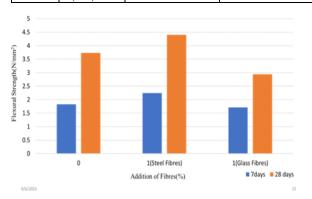
Flexural strength of normal concrete is 1.83 N/mm2 at 7 days and 3.73N/mm2 at 28 days and flexural strength of steel fibres 2.12 N/mm2 at 7 days and 4.46 N/mm2 at 28 days and flexural strength of glass fibres 1.71 N/mm2 at 7 days and 2.94 N/mm2 at 28 days.
