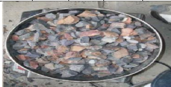
Fig 1 Crushed Over Burnt Bricks
