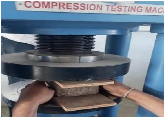
Figure(b): Compression strength test
