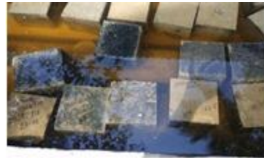
Figure(d): Curing the cubes for 7, 14, & 28 days.
