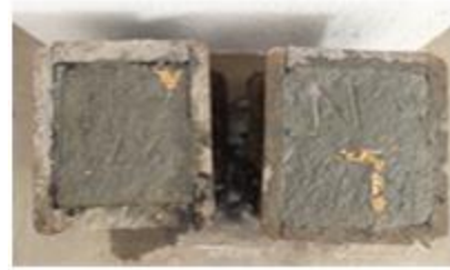
Figure(c): Casting the concrete cubes
