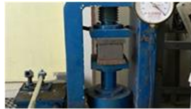
Figure(e): Cubes tested under compressive testing machine.
