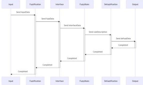
Fig.1. Architecture of Fuzzy system in Artificial Intelligence
