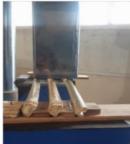
Fig 7. Load testing on platform made up from C section Bamboos
