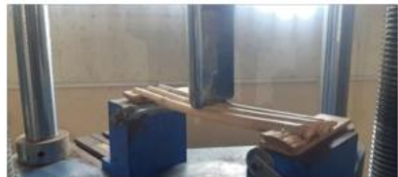
Fig 6. Load Testing on Platform Made from full Bamboos
