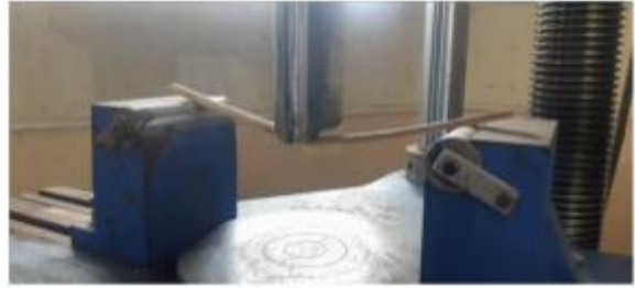
Fig 4. Load testing on Inverted U Section Bamboo
