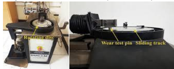
Figure 5: Pin on Disc Wear Testing Machine Carefully interpret results and compare them with relevant standards to assess the material's wear resistance and performance.
