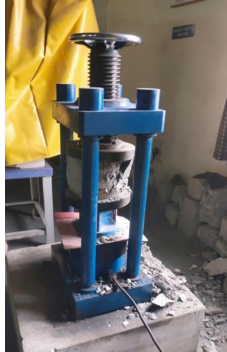
Fig 3: Compressive strength test
