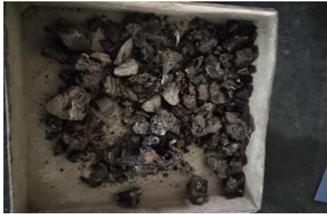
Fig: 1 Sample of steel slag
