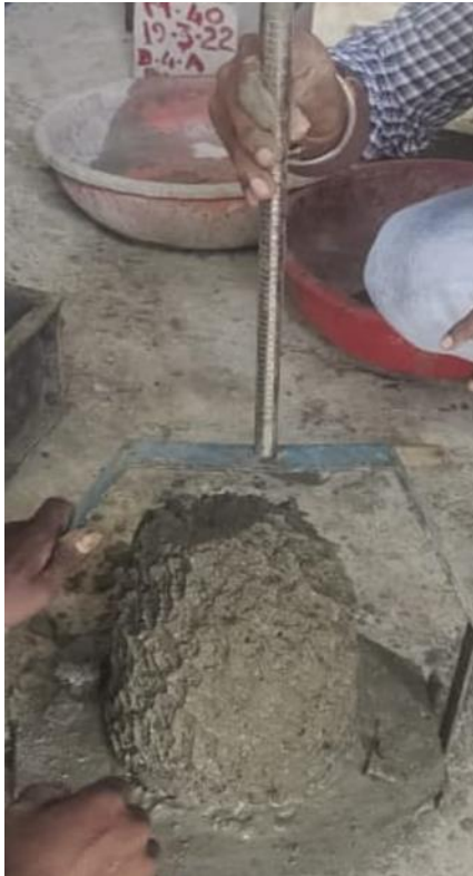
Fig: 2 Slump cone test
