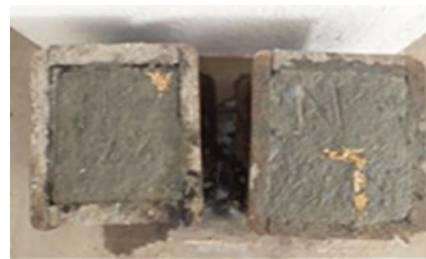
Figure(c): Casting the concrete cubes
