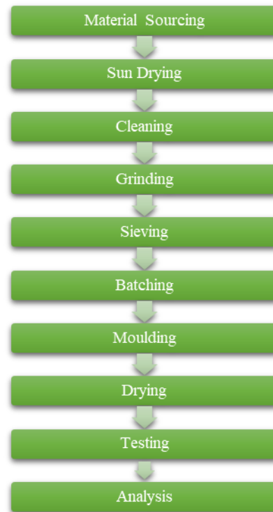
Figure 2: Process of preparation of brick emitting sound absorbing property using agro waste
