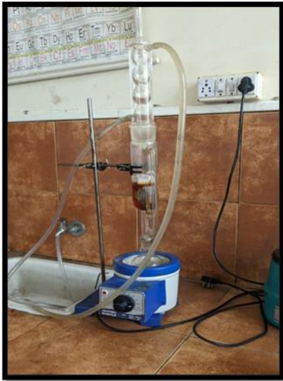
Fig: -1. Extraction Process by using Soxhlet apparatus.
