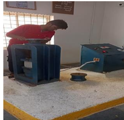
Figure(e): Cubes tested under compressive testing machine.
