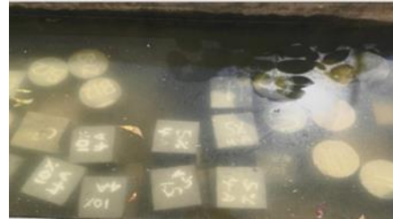
Figure(d): Curing the cubes for 7, 14, & 28 days
