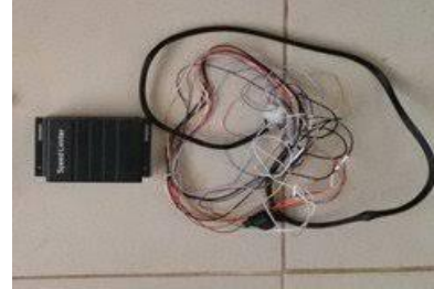
Fig.4 Road Speed Limiter Device and Power Cable
