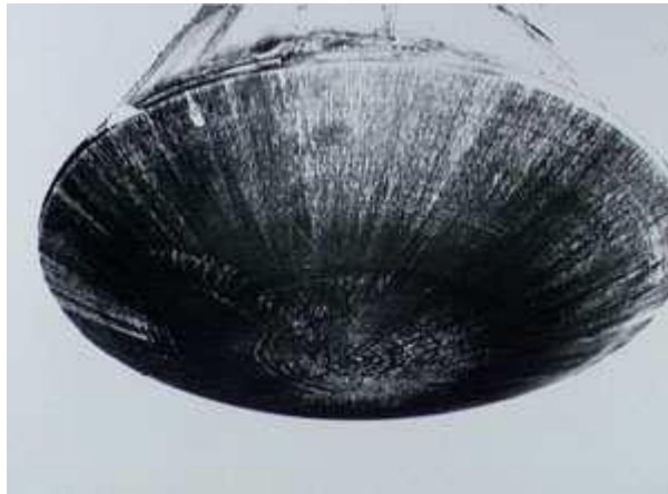
Fig. 1: Mercury spacecraft ablative heat shield after recovery
