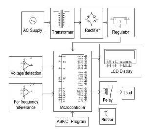
REGULATOR-7805 /7812 gives constant 12 v and 5v.and this voltage applied to the circuit.
