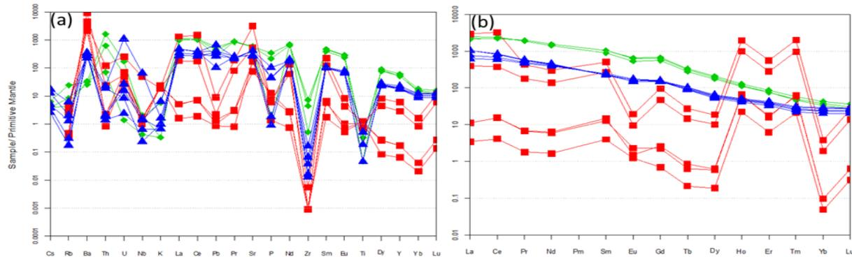
Figure 4. (a) Primitive mantle normalized (after Sun and McDonough, 1989) trace element spiderdiagrams for Hogenakkal carbonatites and other DSRZ carbonatite Complexes. (b) Chondrite normalized (after Boynton, 1984) REE patterns for Hogenakkal carbonatite and other DSRZ carbonatite Complexes.
