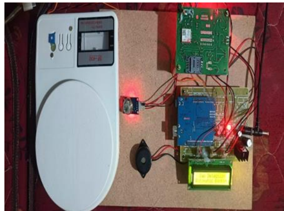
Fig: Gas Monitoring System without Load
