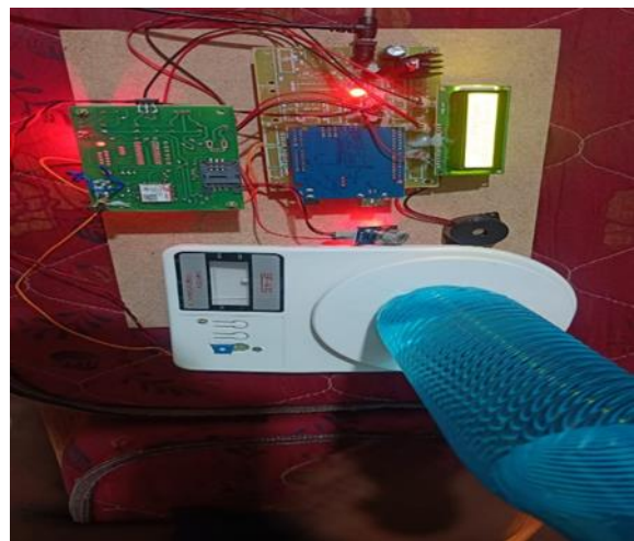
Fig: Gas Monitoring System with Load
