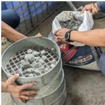
Figure1: - Sieving of Demolished Concrete
