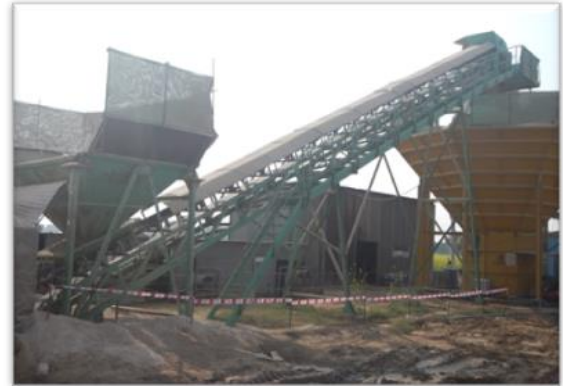
Fig 5 Aggregate bins and conveyor belt for sand and aggregates are not covered to control fugitive dust emissions
