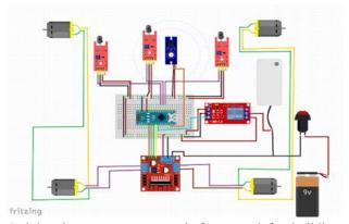
Arduino is an open-source platform used for building electronics projects. Arduino consists of both a physical programmable circuit board (often referred to asa microcontroller) and a piece of software, or IDE (Integrated Development Environment) that runs on your computer, used to write and upload computer code to the physical board.
